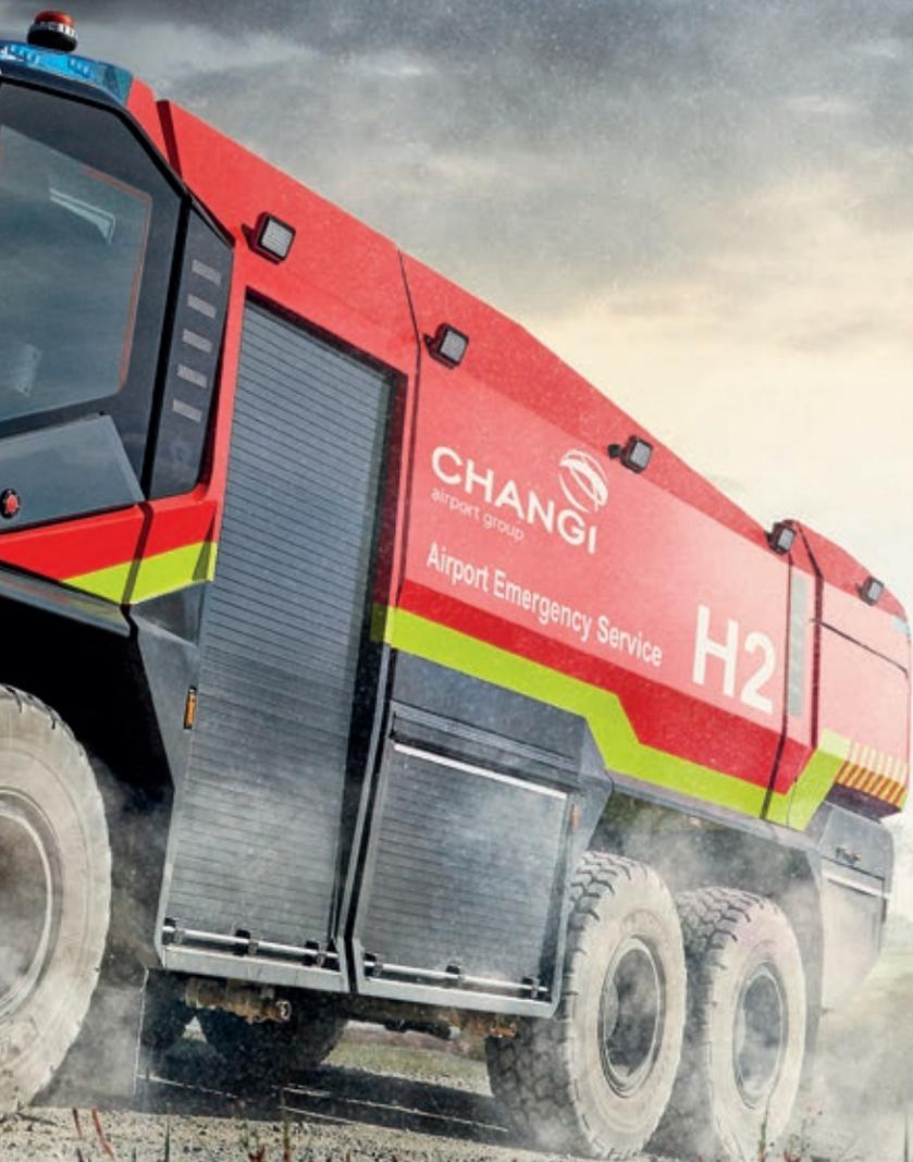
The new PANTHER is available with two different drive variants: basic with Volvo Euro 5 engine and 6-speed gearbox or performance package with Volvo Euro 6 engine and 8-speed gearbox.
