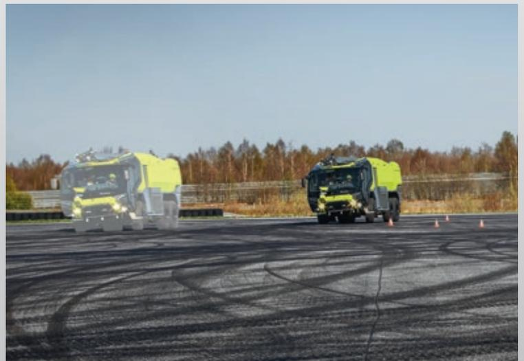
Driving through corners at high speed without / with RSC
