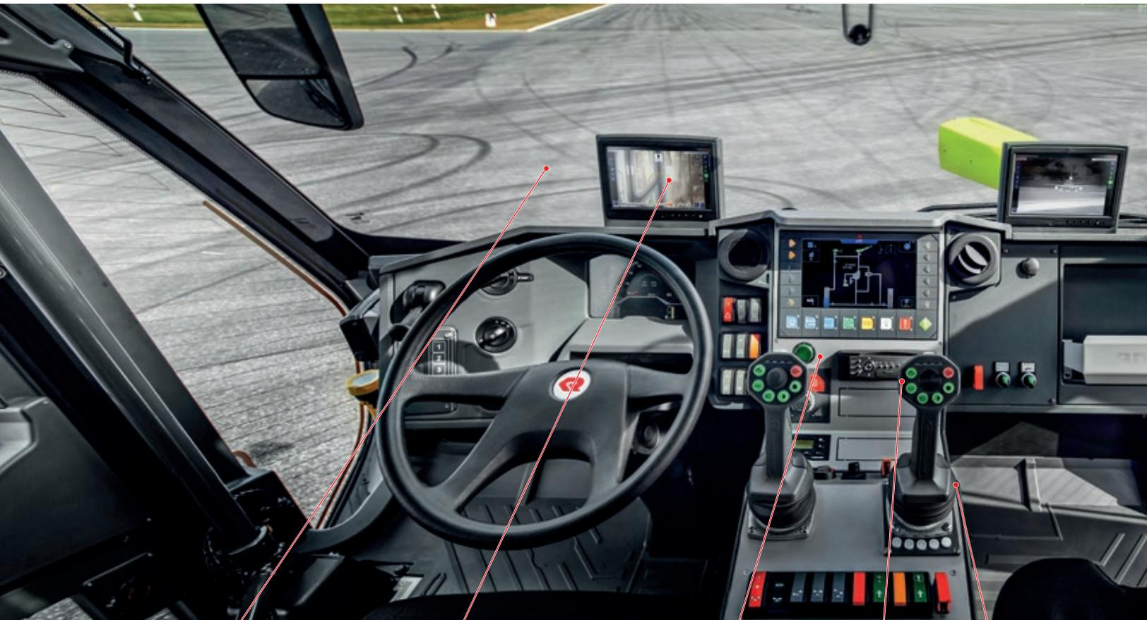
*Integrated additional displays for infrared and color cameras as well as EMEREC DEVS*
